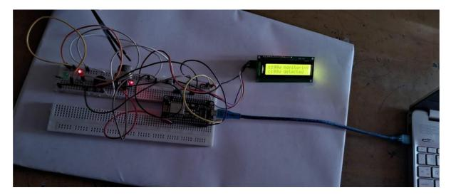
FIG.4 DETECTION OF SMOKE
