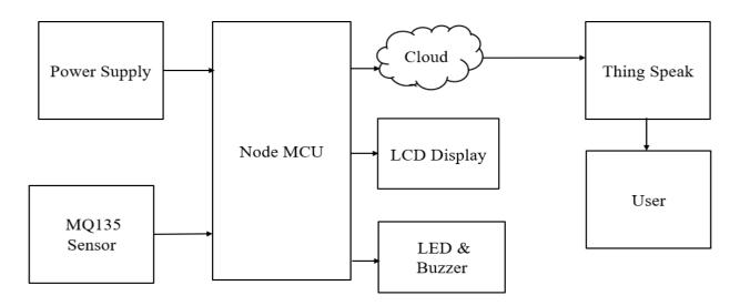
Fig 1. Block diagram for proposed method
